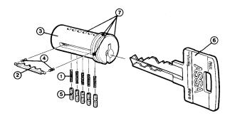
Side bar assembly method is the same for all ASSA Twin 6000 cylinders.
