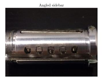
Above is a picture of a sidebar where the front three sliders are set to true gates while the rear two are set to false gates. Note the angle the sidebar is allowed to engage the sliders. This is plenty to allow the lock to open with little resistance.
