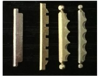
Shown is the sidebar for the CX5 compared to the sidebars from the Schlage Primus, the ASSA Twin 6000, and the Mul-T-Lock MT5+. Note the ridges between the fences, these help align the sidebar as it enters its slot.
