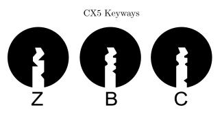
These keyways are not cross-compatible in any way, and, as far as I know, multi-section keys do not exist for them. It appears that a multi-section key could be easily produced for the B and C keyways, however again to my knowledge no such key exists.
