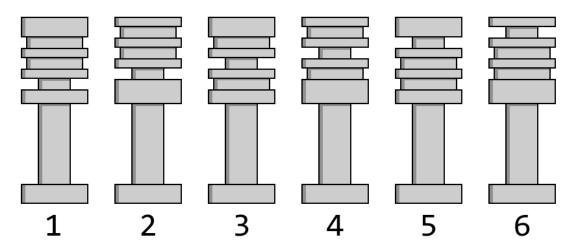
Scale drawing of all six cuts of pin
