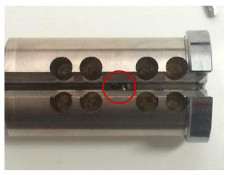
Key retention pins in place within the plug
