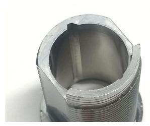
Sidebar grooves inside the housing
